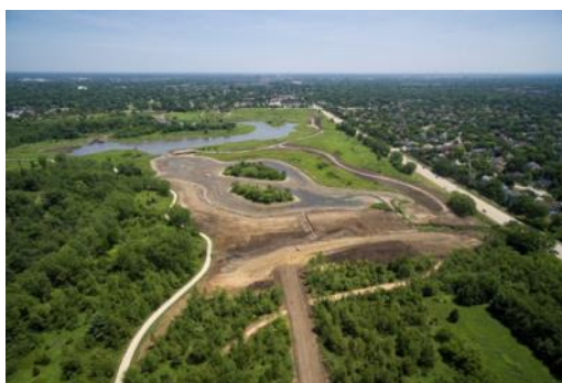
The Buffalo Creek Reservoir Expansion Accomplishes Flood Control, Water Quality Improvement, Natural Restoration, and Active Recreation Objectives Simultaneously
