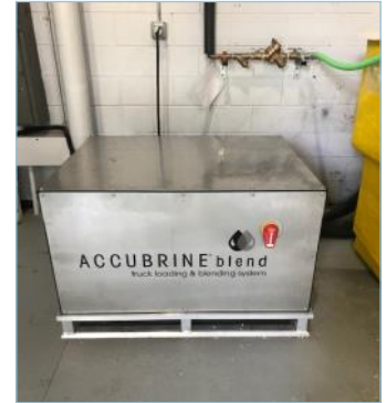
Accubrine – Accubrine unit from Cargill that mixes anti-icing products
