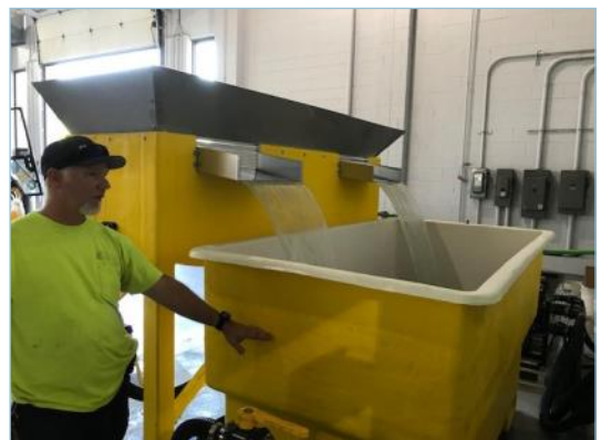
Brine Maker – Maintenance staff member Dave Clauser explains how the Accubrine system works
